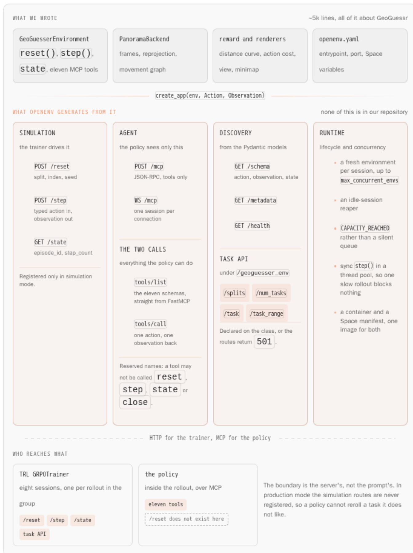
Figure 6 · Orange is what create_app() derives from the environment class. The trainer drives the simulation over HTTP, the policy only ever sees tools over MCP, and in production mode the simulation routes are never registered at all.
